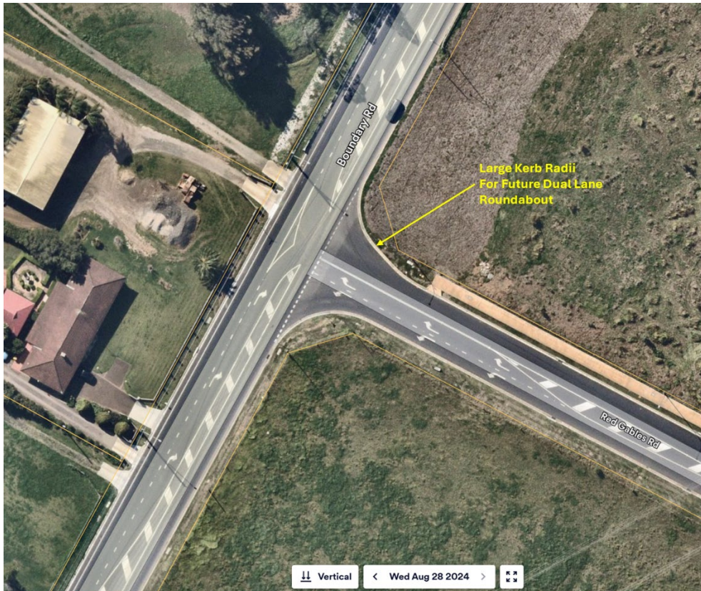
Figure 2 - Large Kerb Radii in Red Gables Road at Boundary Road Rd for Future Dual Lane Roundabout
