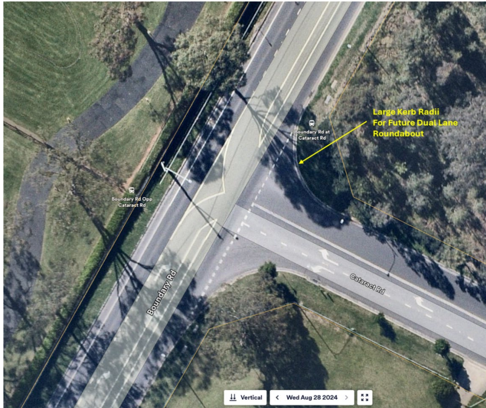
Figure 1 - Large Kerb Radii in Cataract Rd at Boundary Road for Future Dual Lane Roundabout
